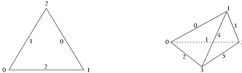
Figure 2.1: Local indices of edges/neighbours in 2d and local indices of edges in 3d.
