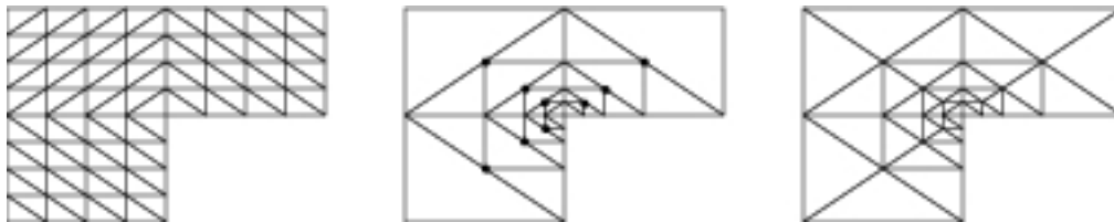
Figure 1.3: Global and local regular refinement of triangles and conforming closure by bisection.
